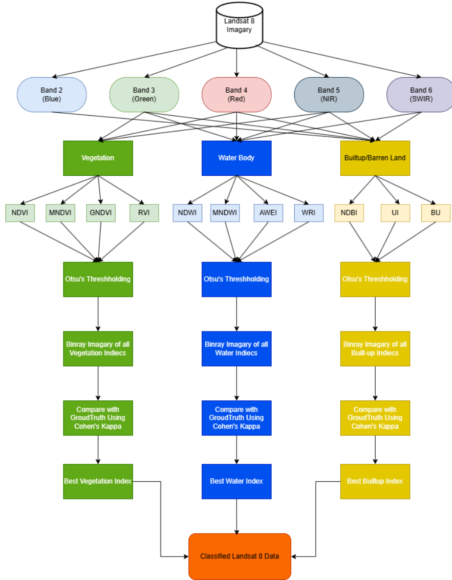
Fig. 2. Methodology workflow for LULC classification using spectral indices
